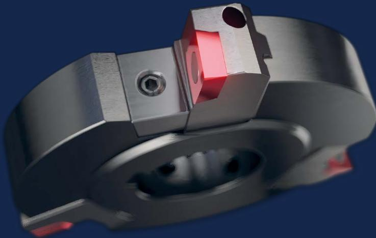
In polygon turning on lathes and multi-spindle machines, peripheral surfaces (shell surfaces) are produced with a fly cutter on the parts to be turned. The workpiece (on main spindle) and the tool (rotating) have to run at an absolutely synchronous transmission ratio.
